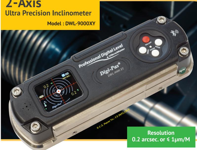
Digi-Pas® DWL-9000XY is a 2-Axis Ultra Precision Inclinometer with built-in Vibrometer, having resolution of 0.2 arcsec. and wide measuring range of 7200 arcsec or 33mm/M for high precision leveling, tilted-plane angles measurements, 2D surface-plane profiling & precision alignment tasks, and capable of real-time wireless Bluetooth/USB remote measuring & data logging when used with PC Sync Software/ Mobile Sync App.
